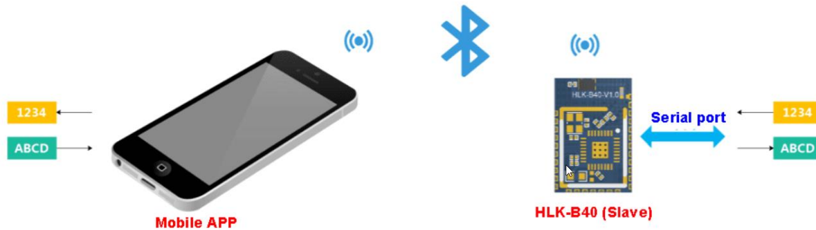
One-to-one Bluetooth connection transmission function schematic
